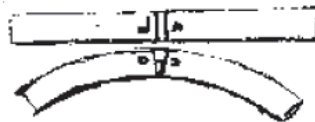
Figure 1.1 Leonardo's description of beam bending [1].
